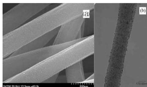
Fig.1 SEM (a) and TEM (b) images of Sm-TiO<sub>2</sub>/CNFs
