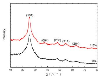
**Fig.2** X-ray patterns of TiO<sub>2</sub>/CNFs and Sm-TiO<sub>2</sub>/CNFs
