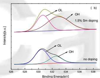
**Fig.3** XPS patterns of O<sub>1s</sub> of TiO<sub>2</sub>/CNFs (no doping) and Sm-TiO<sub>2</sub>/CNFs
