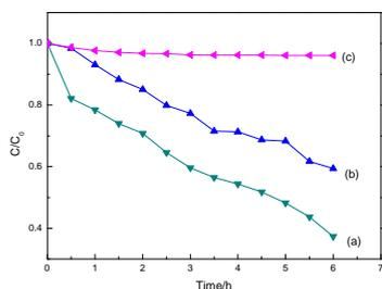
**Fig.4** Photodegradation of methyl orange in the presence of Sm-TiO<sub>2</sub>/CNFs (a), TiO<sub>2</sub>/CNFs (b) and control (c) under UV irradiation
