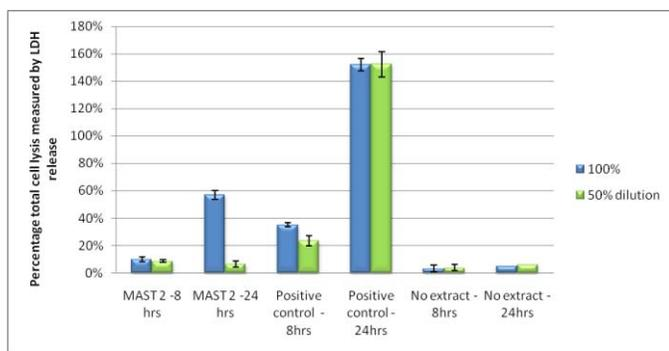
**Fig. 4.** The effect of material extract cytotoxicity after 8 & 24hrs incubation, expressed as percent cell lysis measured by LDH release (mean n=3, +/-sem).
