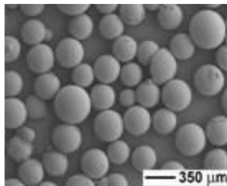
Fig.1 SEM image of MAST 1 beads
