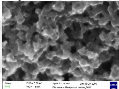
Fig 2. High magnification SEM image of mesoporous domains of MAST 1 (EVO series SEM, Carl Zeiss SMT Ltd).
