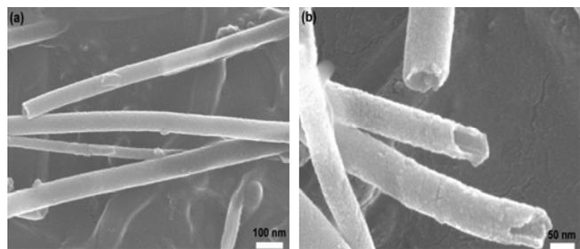
**Fig. 3** SEM images of CNTs etched by HNO<sub>3</sub> with different time (a) 10 h (b) 16 h
