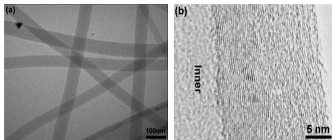
**Fig. 1** Images of as-prepared MWCNTs (a) TEM (b) HRTEM
