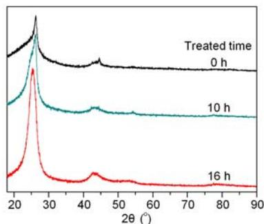
**Fig. 4** XRD patterns of CNTs etched by HNO<sub>3</sub> with different time
