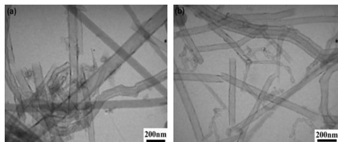
**Fig. 2** TEM images of CNTs etched by HNO<sub>3</sub> with different time (a) 10 h (b) 16 h
