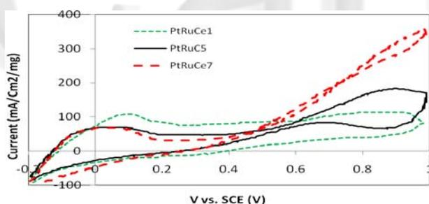
**Fig. 3** Cyclic voltammetric curves of PtRuCe1, PtRuCe5 and PtRuCe7 in 0.5 M H<sub>2</sub>SO<sub>4</sub> containing 1 M methanol.
