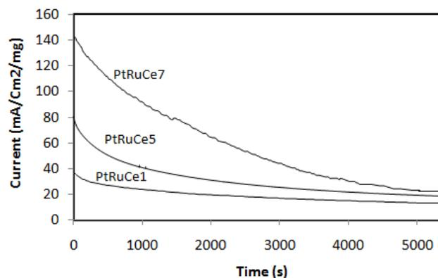
**Fig. 4** Chronoamperometry curves for PtRuCe1, PtRuCe5 and PtRuCe7 in 0.5 M H<sub>2</sub>SO<sub>4</sub>+ 1 M methanol at 0.6 V for 5400 s.
