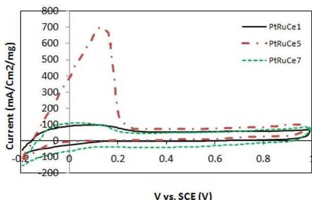
**Fig. 2** Cyclic Voltammograms of PtRuCe1, PtRuCe5 and PtRuCe7 in 0.5 M H<sub>2</sub>SO<sub>4</sub> solution.
