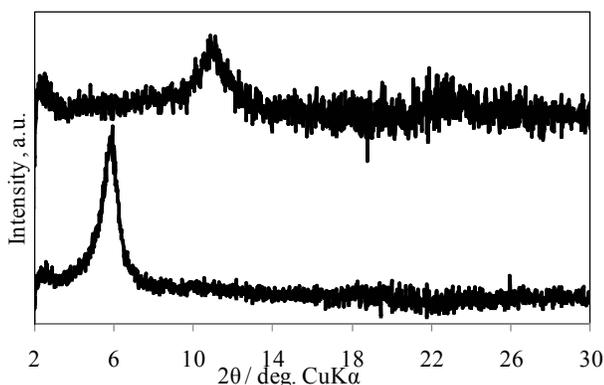
**Fig. 2** X-ray diffraction patterns of  $C_8SiGO$  thin films before and after UV light irradiation for 24h.
