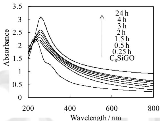
**Fig. 1** UV-Vis spectra of  $\text{C}_8\text{SiGO}$  thin films before and after UV light irradiation.
