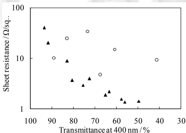
**Fig. 3** Relationship between the transmittance at 400 nm and the sheet resistance of the carbon film obtained from  $C_8SiGO$  film: ○, together with those for  $C_8SiGO$  films heated at 500°C: ▲.
