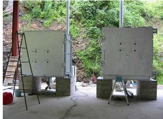
Photo.5 Carbonization furnace by using exhausted gases during carbonization
