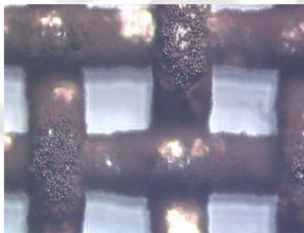
**Figure 3.** Light Microscope Photograph of CMS bonded to a mesh screen (100X)
