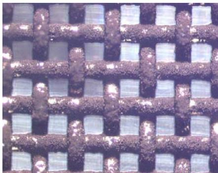
**Figure 2.** Light Microscope Photograph of CMS bonded to a mesh screen (40X)
