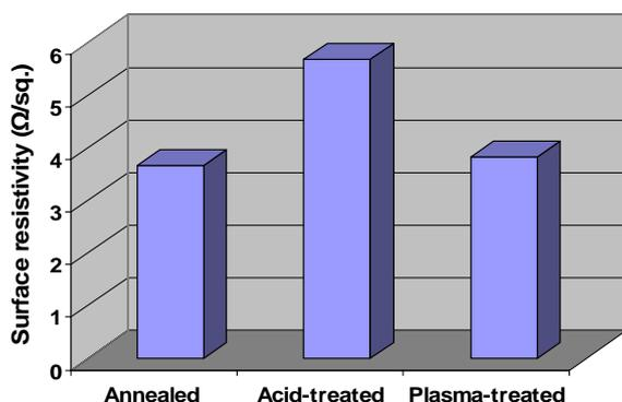
**Fig. 3** Electrical surface resistivity of the buckypapers prepared from annealed, acid and plasma-treated MWCNTs.
