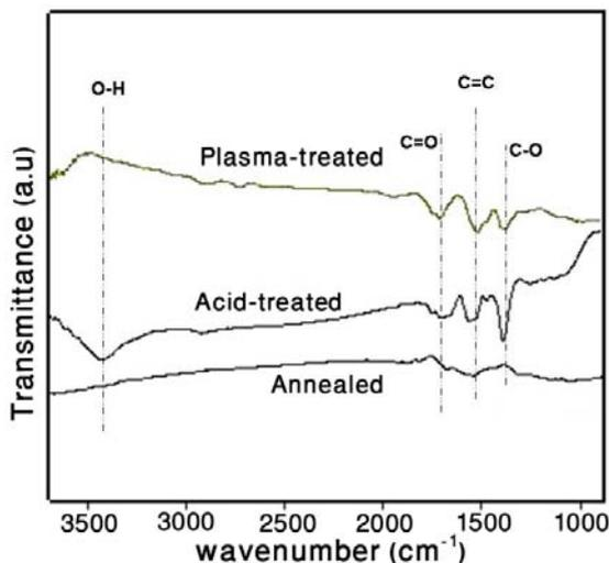
**Fig. 2** The FT-IR spectra of annealed and functionalized MWCNTs.
