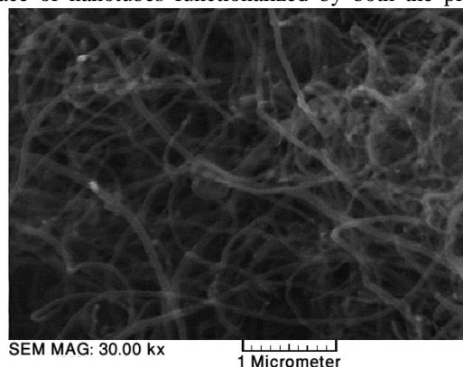
Fig. 1 SEM image of annealed MWCNTs.
