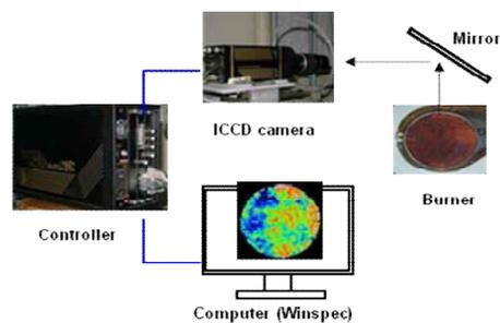
**Fig. 4** Experimental setup for IR spectrum and radical analysis
