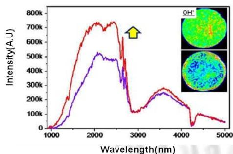
**Fig. 5** IR spectrum and radical analysis of SiC fiber mat during gas radiation test
