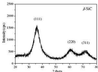
**Fig. 3** X-ray diffraction pattern of SiC mat pyrolyzed the PCS mat derived from preceramic fiber mat at 1200°C for 1 hour
