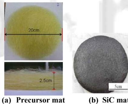
**Fig. 1** Photograph images of (a) preceramic fiber mat (after curing in air) and (b) SiC mat pyrolyzed (a) at 1200°C.
