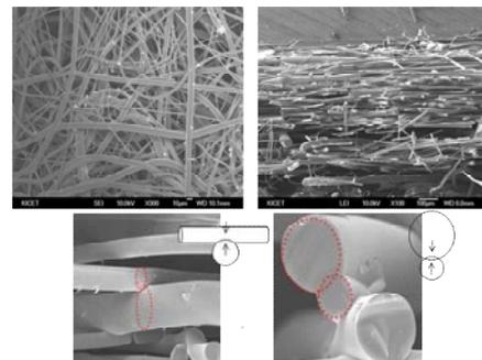
**Fig. 2** FE-SEM images of SiC mat pyrolyzed the preceramic fiber mat pyrolyzed at 1200°C for 1 hour
