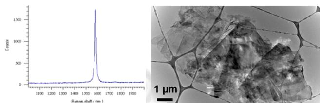
**Fig 4.** Laboratory analogues : carbons obtained by heat-treatment at 1600°C of saccharose-based char and iron; a : Raman spectrum ; b : bright field TEM image.
