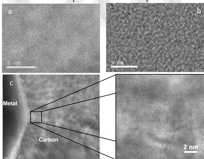
**Fig 3.** Carbon components of the Acapulco meteorite. HRTEM images corresponding to the FIB sections of the figure 2; a: ‘perfect’ graphite, b: ‘imperfect’ graphite, c: preferential orientation of the graphene layers around the iron grain .
