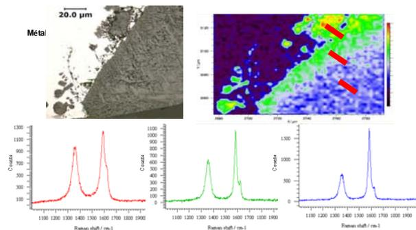
**Fig. 2.** Raman mapping of a carbon inclusion in contact with molten iron; a: optical microscopy image; b: Raman map (the red, green and blue colours correspond to the spectra with increasing the graphitisation degree, and the position of different FIB sections are shown by the red bars).
