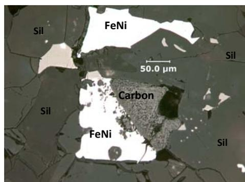
**Fig. 1.** Polished section of the Acapulcoite meteorite as seen by optical microscopy (reflexion mode) and showing the assemblage of silicates, iron-nickel alloys and carbon.
