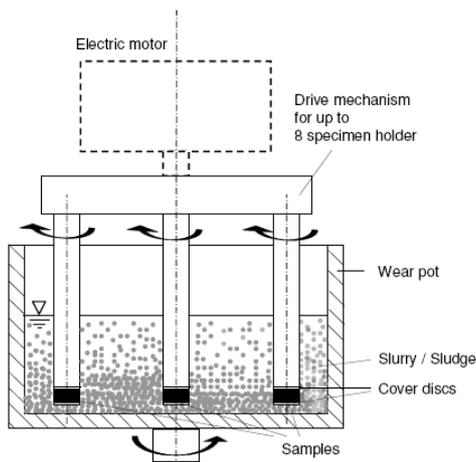
Fig. 1 Principal drawing of test equipment
