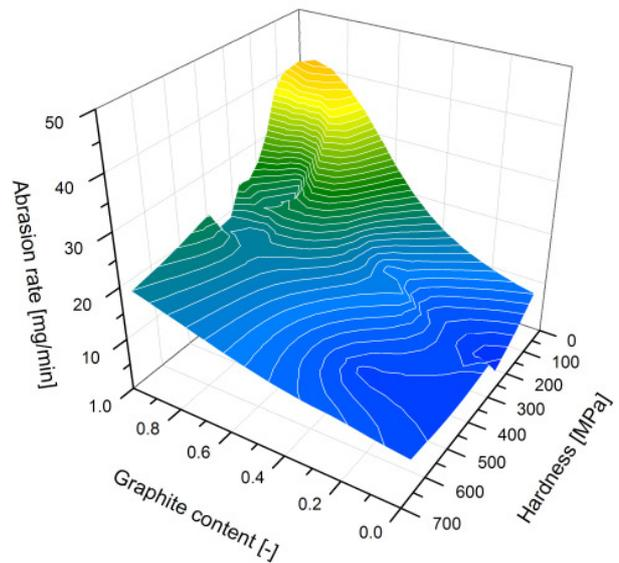
**Fig. 4** 3D-diagram for carbonaceous materials, for visualization of the dependency of slurry-abrasion rates on material hardness and graphite content
