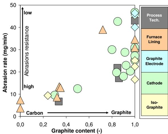
**Fig. 3** Overview of abrasion rates for all 33 materials under investigation, sorted by specific application fields
