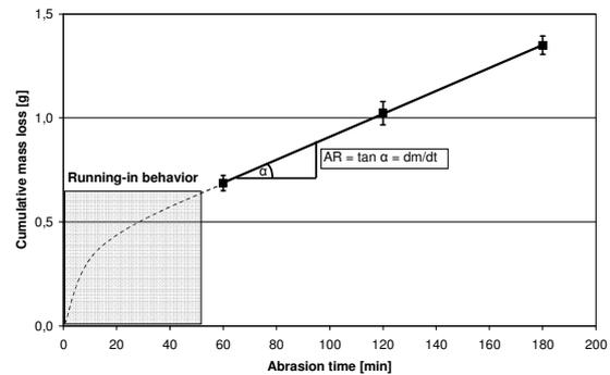
Fig. 2 Exemplary result of a typical slurry-abrasion test with free extrapolation to short abrasion times; error bars reflect one standard deviation
