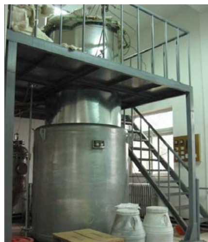
Fig. 4 The pilot plant facility for VACNT array production at a rate of 3.0 kg/h [5].
