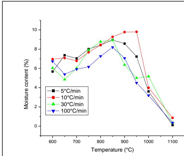
**Fig. 2** – Moisture content as function of carbonizing temperature for fibers treated at different heating rates.
