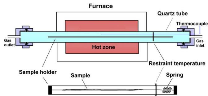
Fig.1 – Carbonization set up used to produce carbon fiber sample from oxidized textile PAN fiber.
