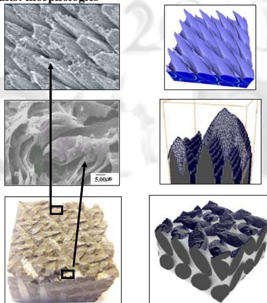
**Fig. 1** Reproduction of the morphological details of a 4D C/C composite ablated in a rocket nozzle test. Left: observed, right: simulated. Top : fiber bundle, mid: pitch-based matrix, bottom: large scale.
