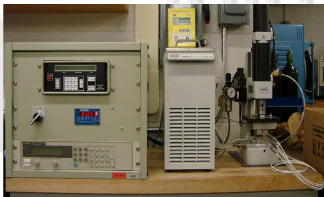
Fig. 2 ASTM D5470 Thermal Impedance Test.
