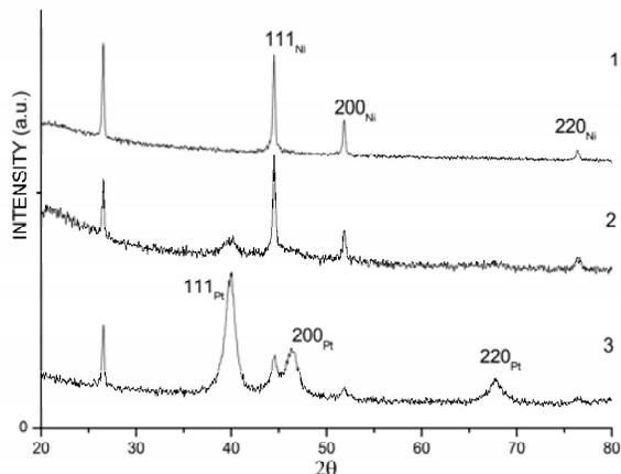
**Fig. 3** X-ray diffraction patterns of carbon encapsulated nickel nanoparticles: after arc discharge (1), after treatment by  $\text{H}_2\text{PtCl}_6$  for 1 h (2) and after treatment by  $\text{H}_2\text{PtCl}_6$  for 4 h (3).
