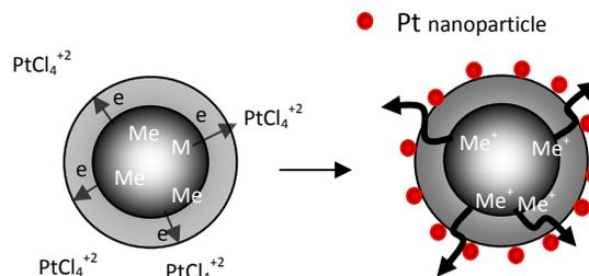
**Fig. 4** Schematic of deposition of platinum nanoparticles during treatment of carbon encapsulated metal by  $\text{H}_2\text{PtCl}_6$  solution.
