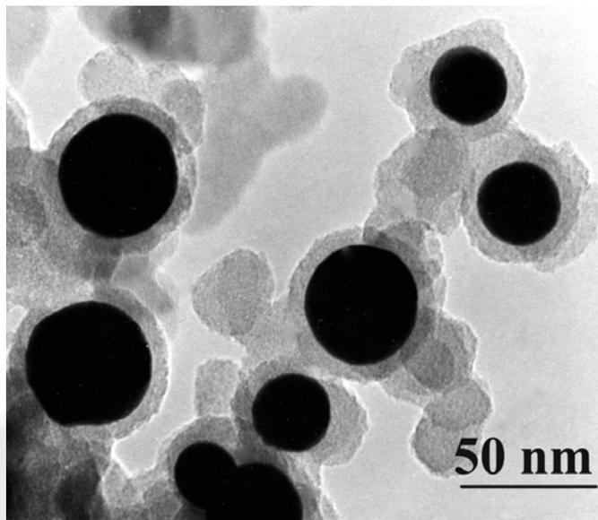
**Fig. 1** Typical TEM images of carbon encapsulated metal nanoparticles.
