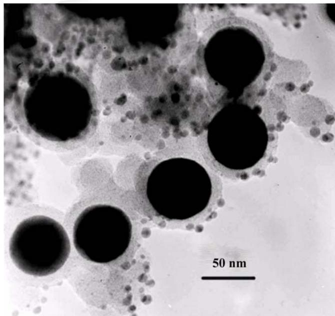
**Fig. 3** TEM image of carbon encapsulated metal nanoparticles after treatment after treatment by  $\text{H}_2\text{PtCl}_6$  solution for 1 h.
