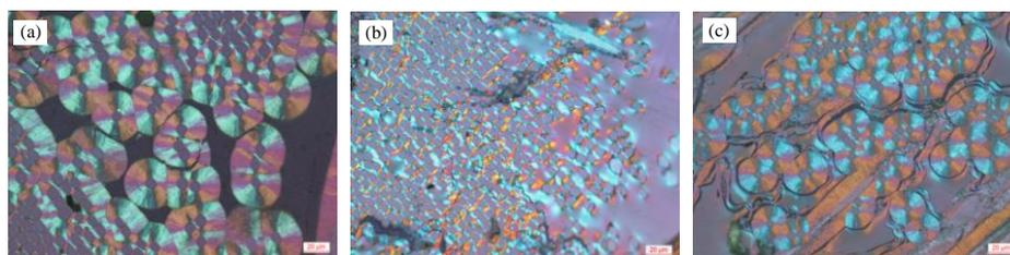
Fig. 1 Characteristic microstructures of C/C composites in PLM. Sampl A (a), sample B (b), and sample C (c).
