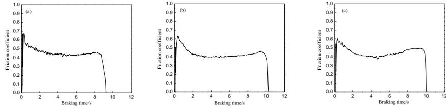
**Fig. 3** Friction coefficient-time curves at 20m/s
