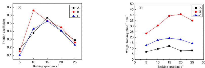
Fig. 2 Relationship between friction properties and braking speeds (a) Friction coefficient-braking speeds curves; (b) Weight loss-braking speeds curves
