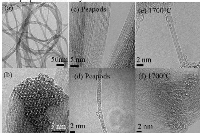
**Fig. 1** TEM images of catalytically grown DWCNTs (a, b) and peapods (c, d), peapods-grown DWCNTs (e, f), respectively.
