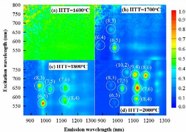
**Fig. 2** Two-dimensional PL maps of the peapod-derived DWCNTs prepared at (a) 1600 °C, (b) 1700 °C, (c) 1800 °C and (d) 2000 °C. The color represents the photoluminescence intensity on a linear scale shown on the right. The open circles show the locations of all peaks, where the values of  $n$  and  $m$  indicate the chirality of the nanotube.
