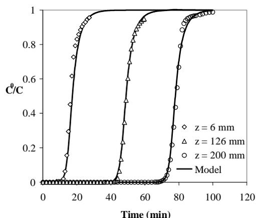
Fig. 2 Modeling breakthrough curves along the adsorber
