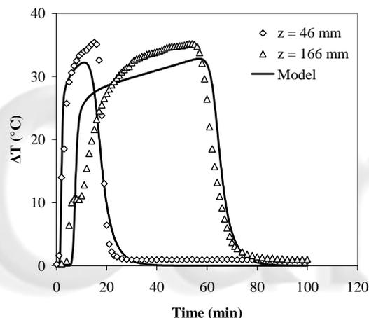
Fig. 3 Modeling temperature profiles along the adsorber
