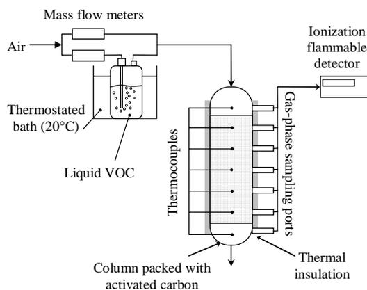
Fig. 1 Schematic of the adsorption column
