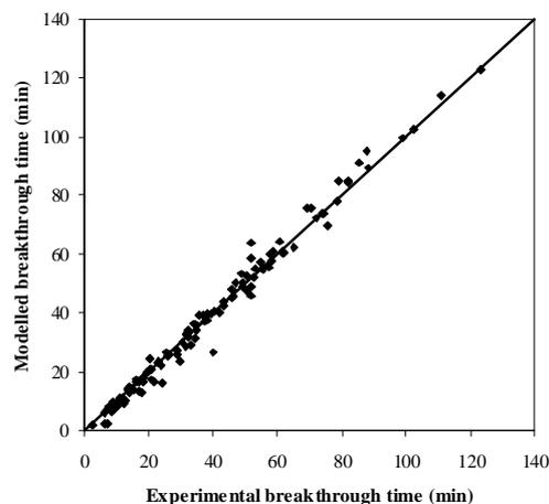
Fig. 4 Results of the simulation – Breakthrough times
