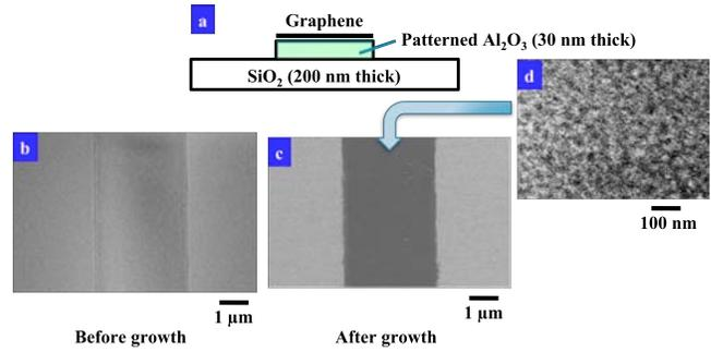
**Fig. 3** (a) Schematic of selective-area growth of graphene on patterned  $\text{Al}_2\text{O}_3$  film. SEM images of a 4- $\mu\text{m}$ -wide line-patterned  $\text{Al}_2\text{O}_3$  film before (b) and after (c) graphene growth. (d) A high-resolution SEM image of the grown graphene on the line-patterned  $\text{Al}_2\text{O}_3$  film.
