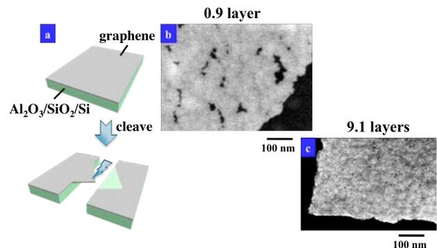
**Fig. 1** (a) Our method to observe the grown graphene on sputtered Al<sub>2</sub>O<sub>3</sub> layer on SiO<sub>2</sub>/Si substrate by a scanning electron microscope (SEM). SEM views of the grown graphene with 0.9 layer (b) and with 9.1 layers (c).
