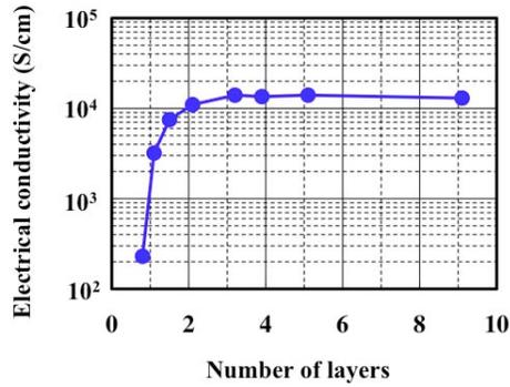
**Fig. 2** Electrical conductivity dependence on the number of layers of graphene
