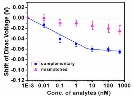
**Fig. 3** The shift of  $V_{g,min}$  for the probe DNA immobilized graphene transistors upon adding various concentrations of complementary or one-base mismatched DNA molecules.
