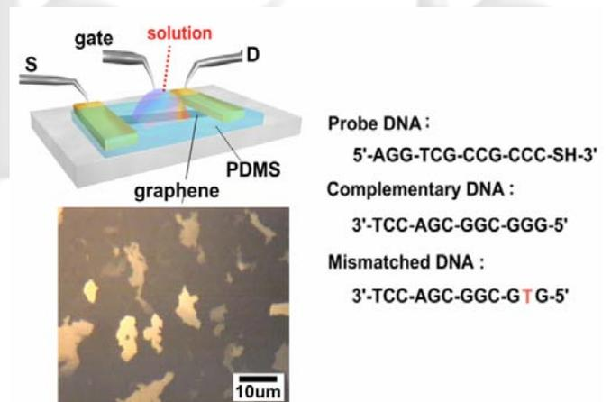
**Fig. 1** Schematic illustration of the graphene device operated by liquid gating. The optical micrograph of the graphene film and the DNA sequences used are also presented .
