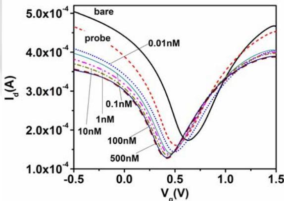
**Fig. 2** Transfer characteristics for the graphene transistors before adding DNA, after immobilization with probe DNA, and after reaction with complementary DNA molecules with the concentration ranging from 0.01 to 500 nM.
