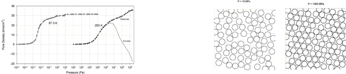
Figure 19: (a) Comparison between sub-critical adsorption at 87.3 K and supercritical adsorption at 253 K (b) Snap shots of argon in 6.5 Å slit pore at 253 K ( P = 1, 10, 1000 \text{ MPa} )
