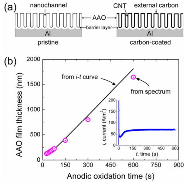
**Figure 1.** (a) Schematics of the pristine AAO film and the carbon-coated one. (b) AAO film thickness estimated from the  $i-t$  curve (inset) recorded during the anodic oxidation.
