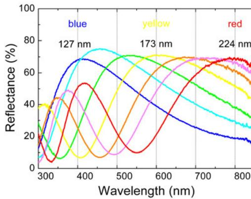
**Figure 3.** UV-vis diffuse reflectance spectra of the carbon-coated AAO films showing interference colors varying from blue to red. The AAO film thickness ranges from 127 nm to 224 nm.
