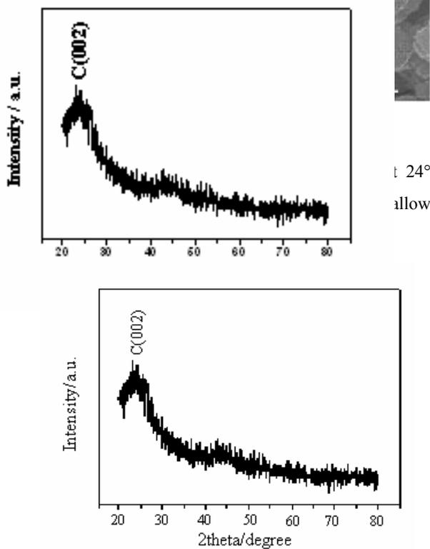
Fig.2 a) High magnification and b) XRD spectrum showing details of the carbon spheres at 40A.
