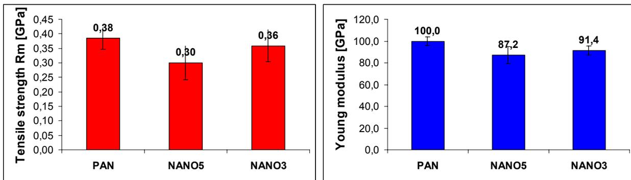
**Figure 1,2.** Mechanical properties of PAN-based and nanotubes – containing PAN-based carbon fibers after carbonization process at 1000°C.
