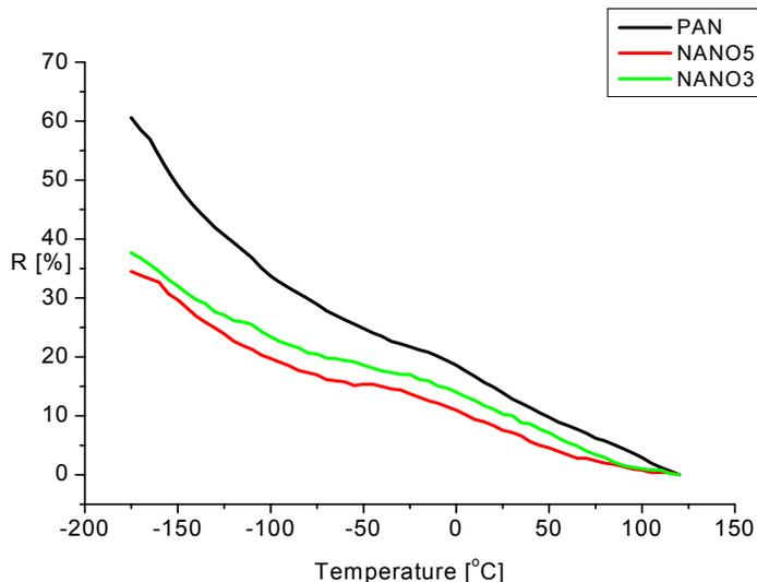
**Figure 5.** Relative resistance changes versus temperature for pure and modified carbon fibers.
