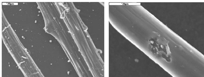
**Figure 3,4.** SEM microphotograph of carbon fibers containing carbon nanotubes.
