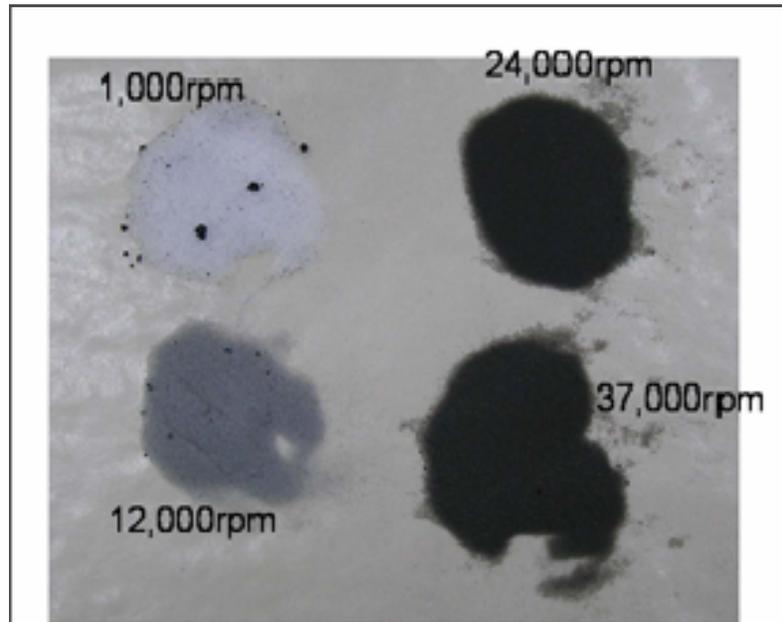
**Figure 1.** Optical microscope images of mixed powders (PMMA+VGCF) mixing at various rotation rate (1,000-37,000 rpm) in 120sec.
