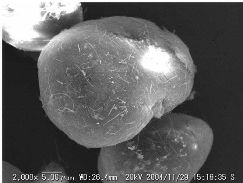
**Figure 2.** SEM image of direct mixed polymer/VGCF powder.
