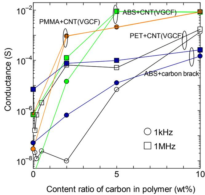
Figure 3. AC conductance of the samples measured at 1kHz and 1MHz.
