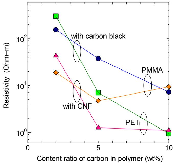
Figure 4. DC resistivity of the samples measured by 4-probe method.
