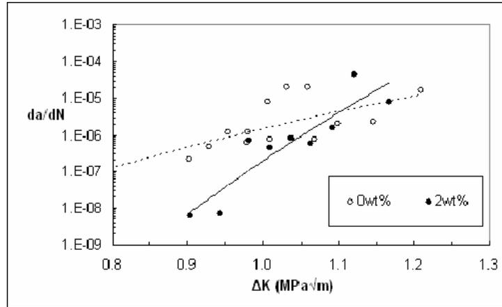
**Figure 1.** The rate of crack growth ( $da/dN$ ) plotted against increasing stress intensity factors ( $\Delta K$ ).
