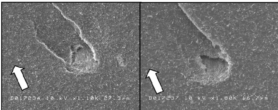
**Figure 2.** SEM micrographs revealed the presence of MWCNT agglomerations. The white arrows indicate the direction of crack growth. The agglomerates likely accelerated the rate of crack growth.
