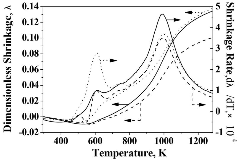
Fig. 5. Comparison of typical dilatometric results. — pure oxidized MP, ..... MWNTs concentration: 5 %, - - - MWNTs concentration: 20 %; Heating rate: 1 K/min in argon.
