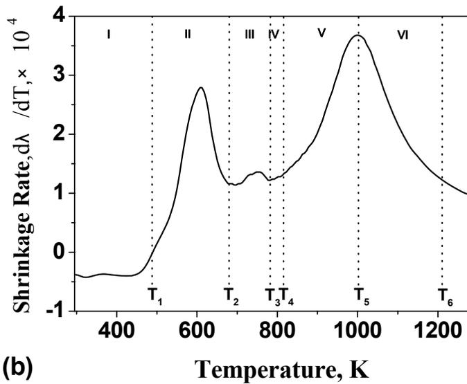
Fig. 4. Typical sample shrinkage during sintering: (a) dimensionless shrinkage  $\lambda$ , as a function of temperature, (b)  $d\lambda/dT$ ; MWNTs concentration: 5 %, heating rate: 1 K/min in argon.
