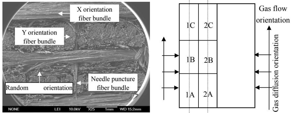
Fig. 1 The image of 2D needle-punched fiber felt
