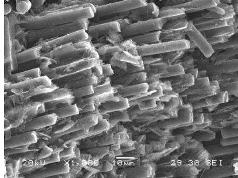
**Fig.5** SEM photographs of fracture surface of mesophase pitch-based C/C composites
