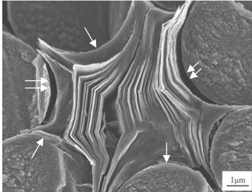
**Fig.2** Original SEM micrographs of mesophase pitch-based C/C composites
