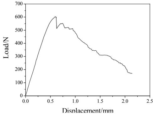
**Fig.4** the curve of load-displacement of mesophase pitch-based C/C composites
