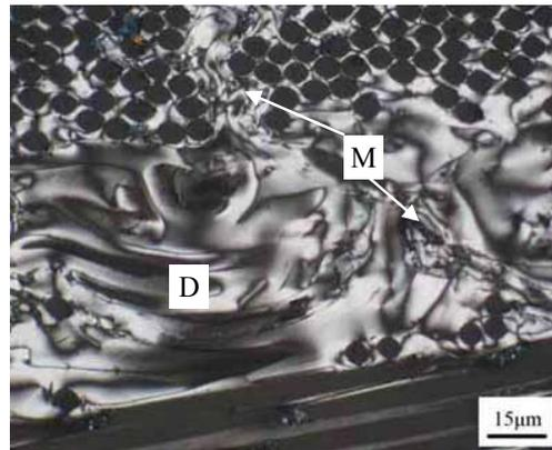
**Fig.1** Polarized light micrographs of mesophase pitch-based C/C composites ----M: mosaic-type pitch matrix; D: domain-type pitch matrix
