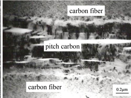
**Fig.3** Low magnification TEM micrographs of mesophase pitch-based structure [8].
