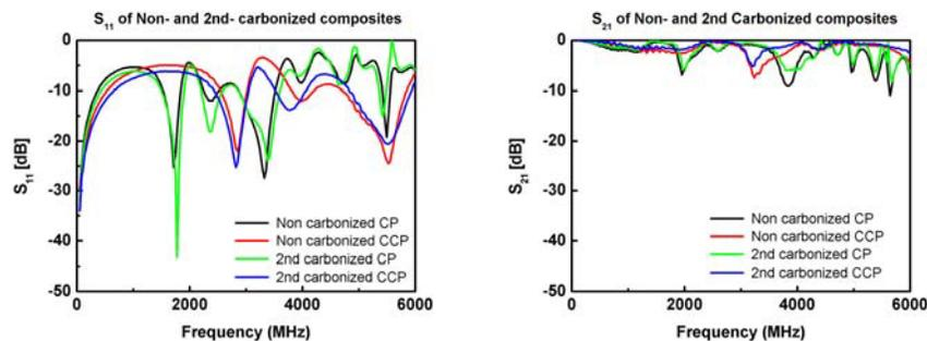
Figure 2.  $S_{11}$  and  $S_{21}$  of Non-carbonized composites and 2<sup>nd</sup> carbonized composites
