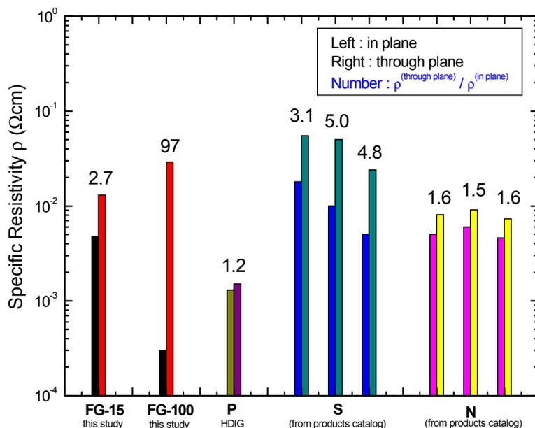
Fig. 2 Anisotropy in electrical resistivity of various carbonaceous bipolar plate
