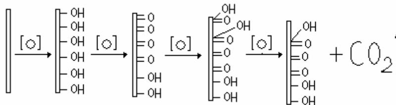
**Figure 2.** Oxidation mechanism of CF
