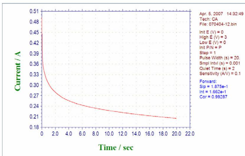
**Figure3.** CA curve of electrochemistry oxidation in 0.5mol/L nitrate electrolyte
