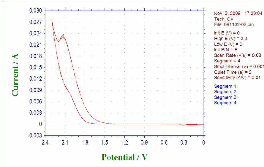
**Figure 1.** CV curve of CF electrochemistry oxidation in 0.5mol/L nitrate electrolyte
