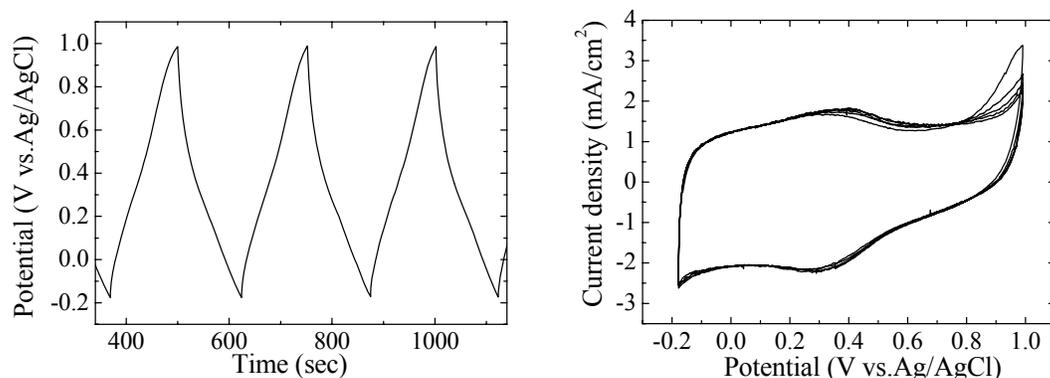
**Figure 1.** Galvanostatic charge/discharge curves (left) and cyclic voltammograms (right) of B/C material prepared by the reaction of cellulose and BCl<sub>3</sub>. Electrolyte : 1M-H<sub>2</sub>SO<sub>4</sub> aq.
