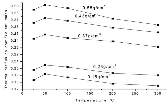
Fig 3: The changes of thermal diffusion coefficient of the carbon foams prepared with temperature change
