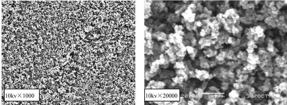
Fig1: SEM microphotographs of phenolic carbon foam with  $0.37\text{g/cm}^3$
