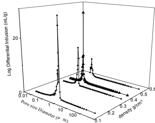
Fig 2: The pore texture of these carbon foams prepared
