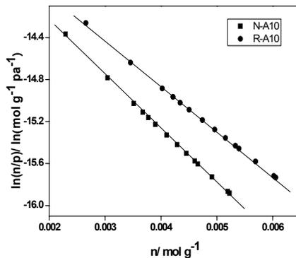
Figure 3. Virial graphs for the adsorption of hydrogen on activated carbon fibers at 77 K.
