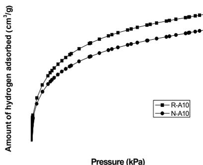
Figure 2. Hydrogen adsorption isotherms of activated carbon fibers used in this study.
