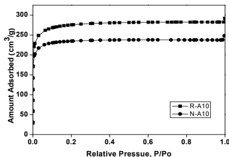
**Figure 1.** Nitrogen adsorption isotherms of activated carbon fibers used in this study.
