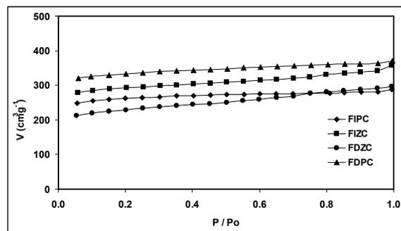
Figure 1.  $\text{N}_2$  Adsorption Isotherms at 77 K
