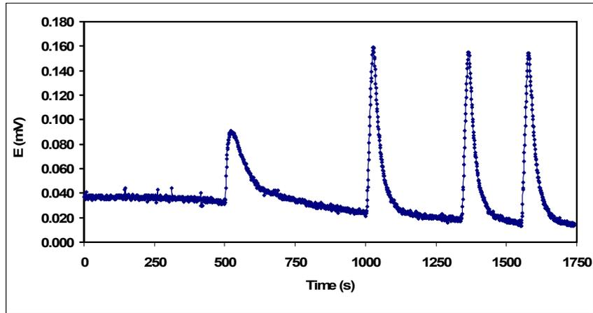
Figure 4. Immersion thermogram of one of the activated carbon fibers in NaOH solution
