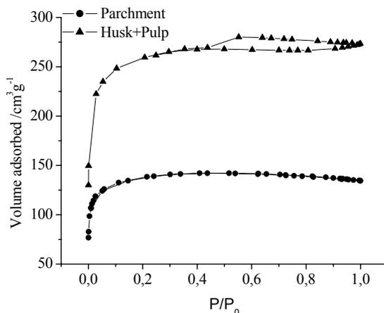
**Figure 2.** Nitrogen adsorption-desorption isotherm of PC and HP activated carbons.
