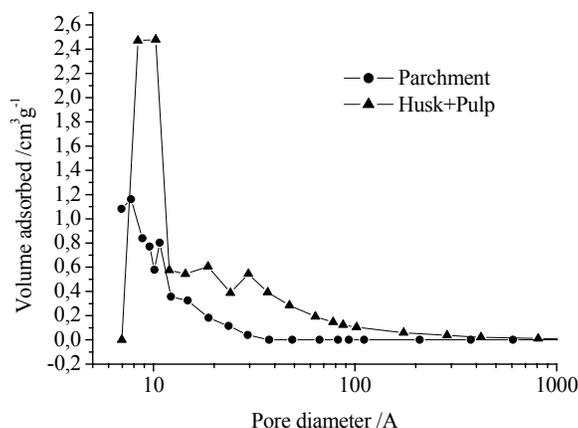
**Figure 3.** Porous size distribution of coffee parchment (PC) and husk+pulp (HP) activated carbon
