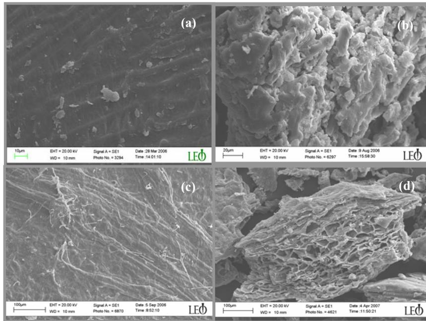
**Figure 6.** SEM micrographs of: (a) PC, (b) PC activated carbon, (c) HP, (d) HP activated carbon.
