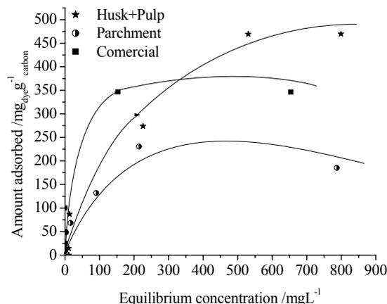
**Figure 7.** Absorption isotherms, at room temperature, of the methylene blue dye on the activated carbons.
