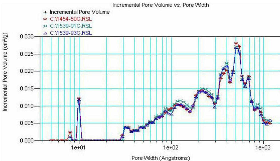
**Figure 2.** DFT Plot of 50 Micron GPC (3 batches)
