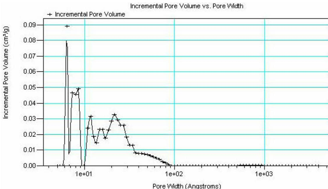
**Figure 1.** DFT Plot of 20-50 Micron CMS
