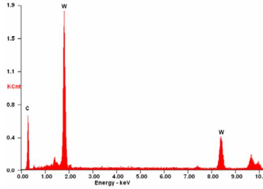
**Figure 3.** EDS analysis of W threads in sample A
