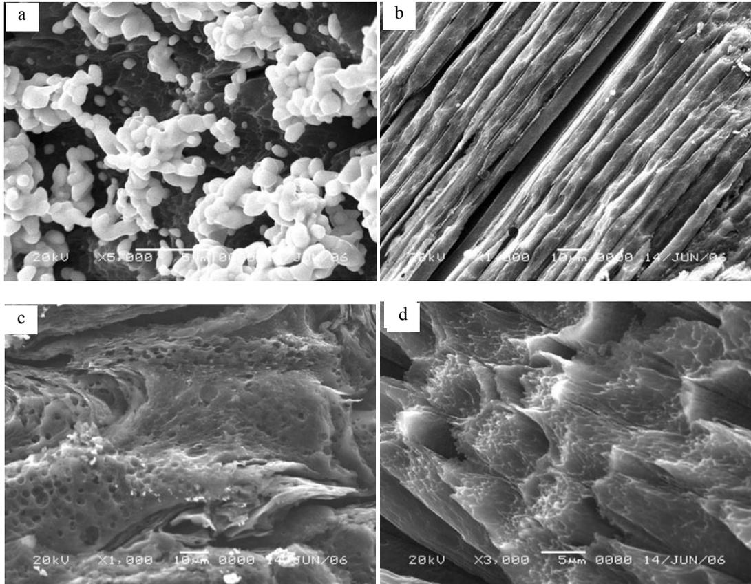
**Figure 7.** Micro-ablation morphologies of sample A
