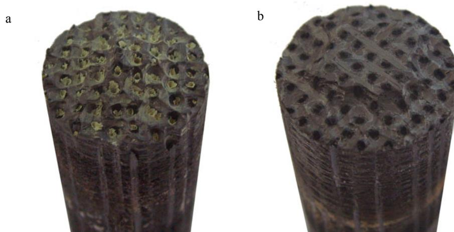
**Figure 5.** Macro-ablation morphologies of sample A and B
