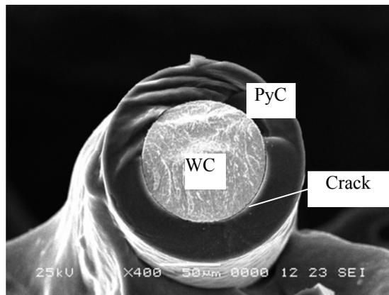
**Figure 2.** Cross-section of one single W thread after CVD
