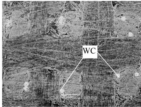
**Figure 4.** Distribution of WC threads in C/C composites
