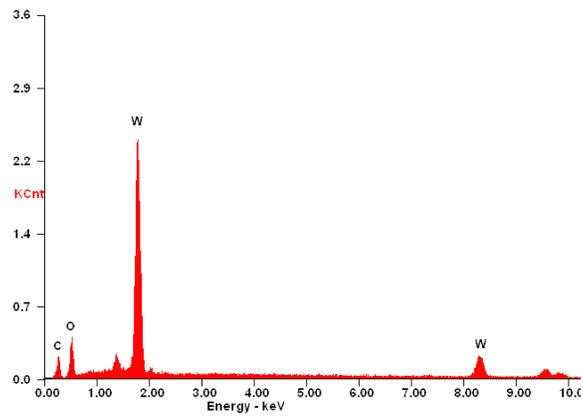
**Figure 8.** EDS analysis of ablation surface of sample A
