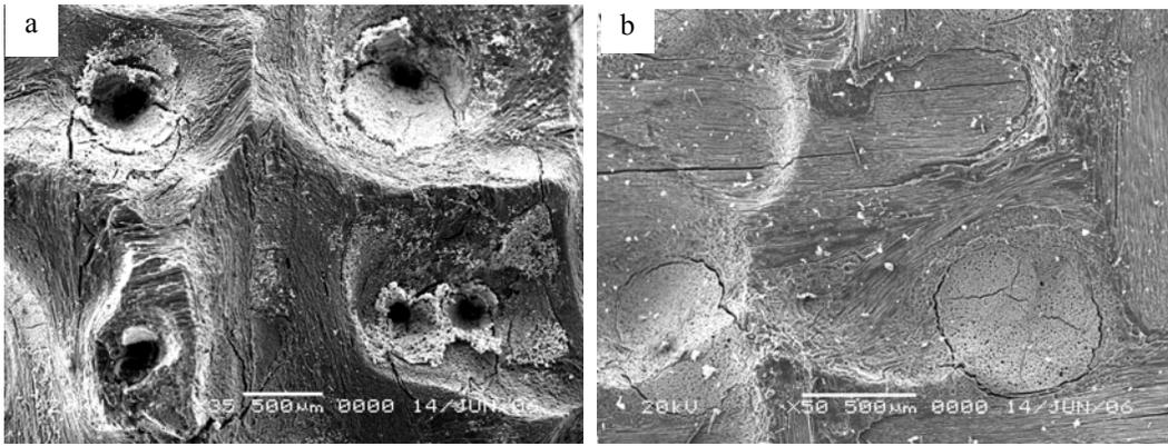
**Figure 6.** Macro-ablation morphologies of sample A and B
