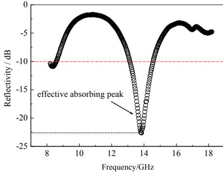
**Figure 6.** Reflectivity vs frequency curve of a standard cement-sand sample without any carbon fibers
