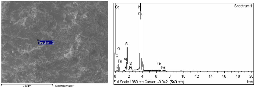
**Figure 2.** SEM image of the fracture surface of a standard cement-sand sample and corresponding EDS graphics
