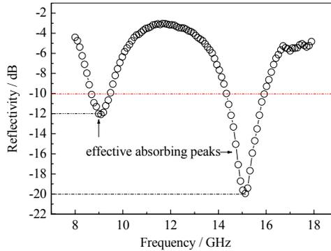
**Figure 7.** Reflectivity as a function of frequency for a fiber mass fraction of 0.2 %
