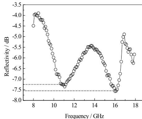
**Figure 11.** Reflectivity as a function of frequency for a fiber mass fraction of 1.0 %
