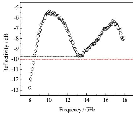
**Figure 10.** Reflectivity as a function of frequency for a fiber mass fraction of 0.8 %
