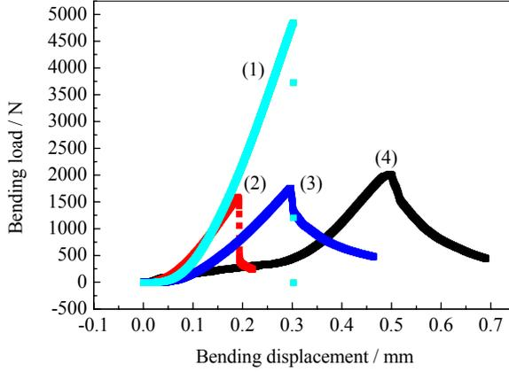
**Figure 5.** Relationship between bending load and displacement of CFRC samples
