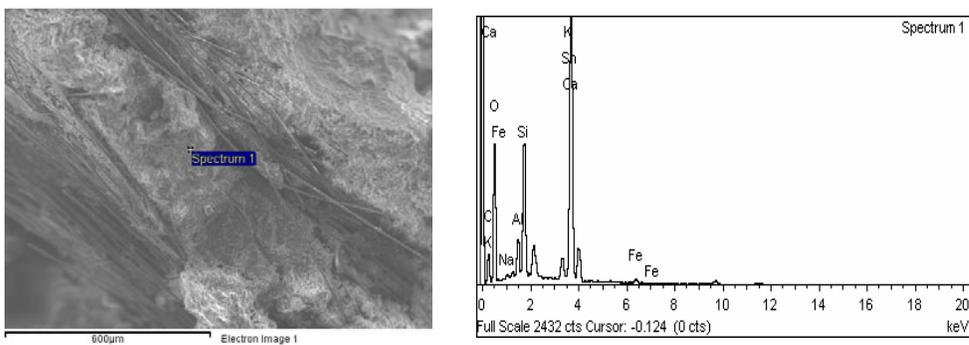
**Figure 4.** SEM image of the fracture surface of a CFRC sample and corresponding EDS graphics for poor dispersion of carbon fibers in the cement matrix
