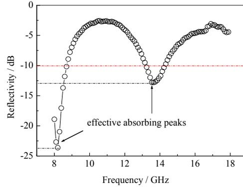
**Figure 9.** Reflectivity as a function of frequency for a fiber mass fraction of 0.6 %
