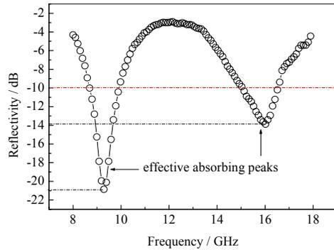
**Figure 8.** Reflectivity as a function of frequency for a fiber mass fraction of 0.4 %
