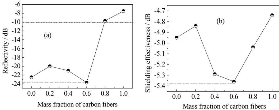
**Figure 12.** Reflectivity as a function of fiber mass fraction (a) and SE as a function of fiber mass fraction (b)
