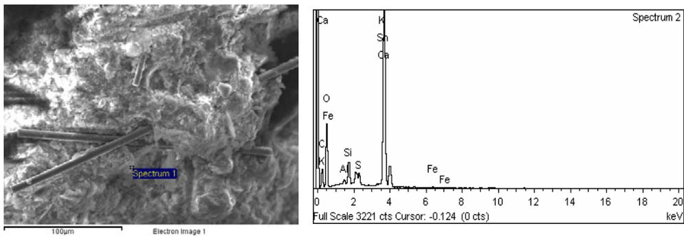
**Figure 3.** SEM image of the fracture surface of a CFRC sample and corresponding EDS graphics for good dispersion of carbon fibers in the cement matrix
