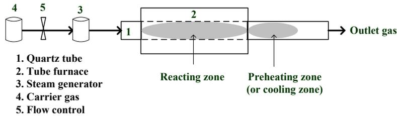
Figure 1. Experimental apparatus in activation
