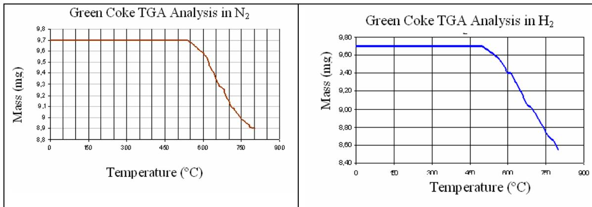
Figure 2. TGA of CV in  $N_2$  and  $H_2$  Atmospheres.
