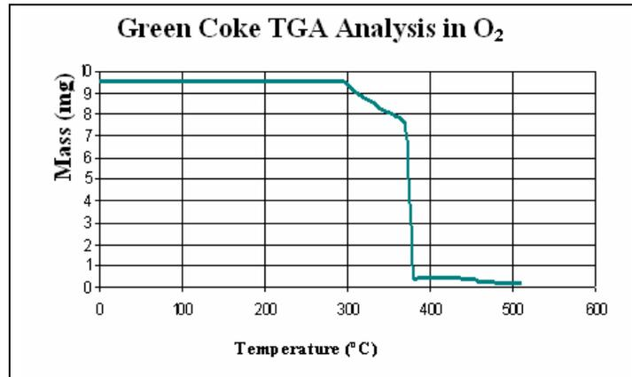
Figure 1. TGA of CV in  $O_2$  Atmosphere.
