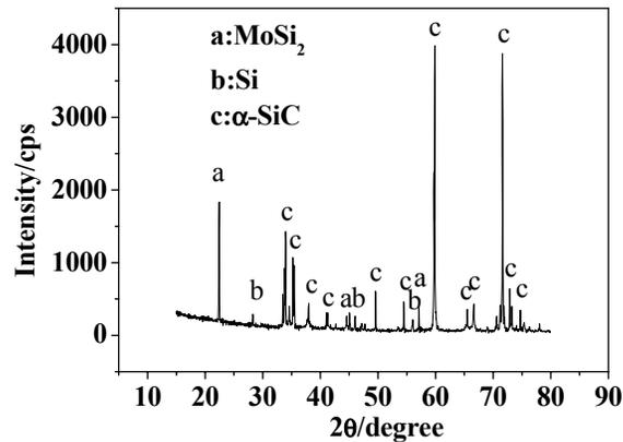
Figure1. X-ray patterns of the coating obtained by two-step pack cementation technique.
