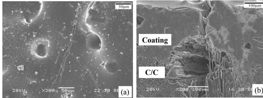
Fig.7 Surface (a) and cross-section (b) SEM images of the MoSi<sub>2</sub>-SiC-Si coated sample after oxidation at 1773K in air for 200h.
