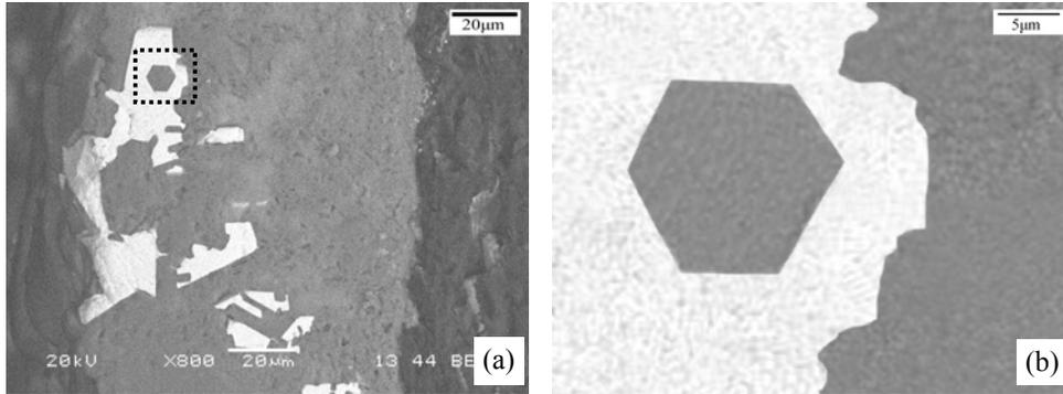
Figure 5. The cross-section backscattering electron image of the coating.
