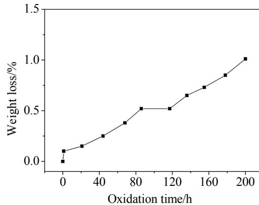
Figure 6. The 1773K isothermal oxidation curves of the coated C/C in air.
