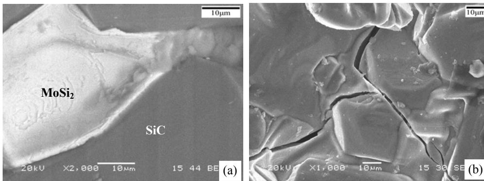
Figure 4. SEM images of the phase interface between MoSi<sub>2</sub> and SiC.
