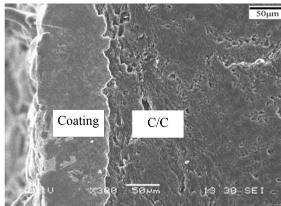
Figure 3. Cross-section SEM image of the coated samples.
