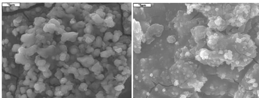
Figure 5. SEM micrographs of surfaces of carbon-phosphate composites modified with natural and synthetic hydroxyapatite after incubation in SBF.
