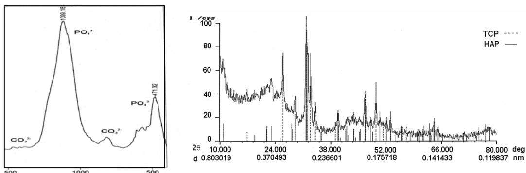
Figure 6 . FTIR and XRD of carbon-phosphate composite CC-HAp(sm).
