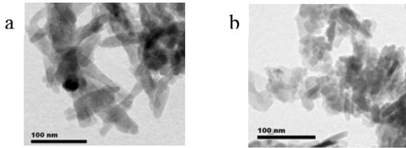
Figure 1. TEM microphotographs of hydroxyapatite powders a) HAp-sn, b) HAp-nn
