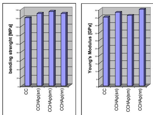
Figure 4. Mechanical properties of carbon-phosphate composites.
