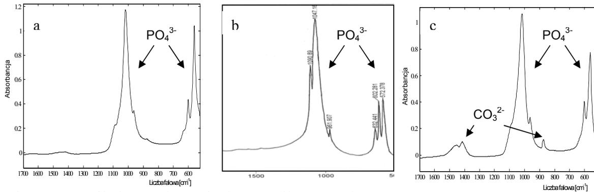
Figure 2. FTIR of hydroxyapatite powder a) HAp-sn, b) HAp-sm, c) HAp-nn.
