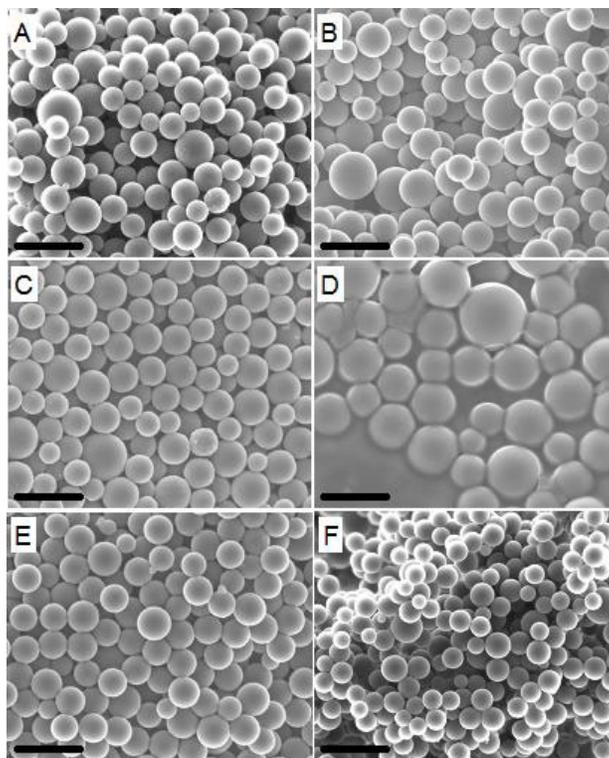
**Figure 1.** SEM images of surface modified LC-derived carbon nanoparticles. (A) As prepared carbon nanoparticles from 0.5 wt-% precursor solution; (B) after sterilization at 400 °C for 15 min in nitrogen flow; (C) after sulfonation at 70 °C for 1 hour; (D) after PLL loading (C:PLL = by weight); (E) after PEG loading (C:PEG = by weight); and (F) after annealing at 1000 °C for 2 min in nitrogen flow. The scale bar: 1 micron.
