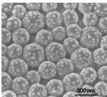
**Figure 6.** SEM image of LC-derived carbon nanoparticles from 0.5 wt-% precursor solutions doped with Se nanoparticles.
