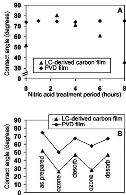
**Figure 2.** Water contact angles on carbon model films after nitric acid treatment and ozone treatment.
