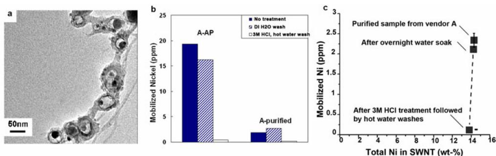
**Figure 5.** Reduction in Ni bioavailability through post-processing. A. TEM image of as-produced SWNT from vendor A after 48hr HCl wash; b. Nickel mobilization of AP and Purified SWNT from vendor A in PSF for different post-treatments; c. The residual free nickel remaining after the original vendor purification process can be greatly reduced by treatment with 3 M HCl and hot water washing. Values are mean  $\pm$  s.e. (shown on or adjacent to point) in pH 5.5 buffer.
