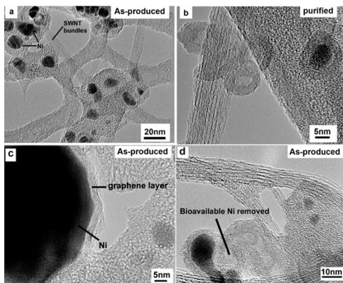
**Figure 1.** Typical morphologies for Ni-containing commercial SWNTs. a, c: As-produced from vendor C; Fig. 1d and 1b are as-produced and purified from vendor A.
