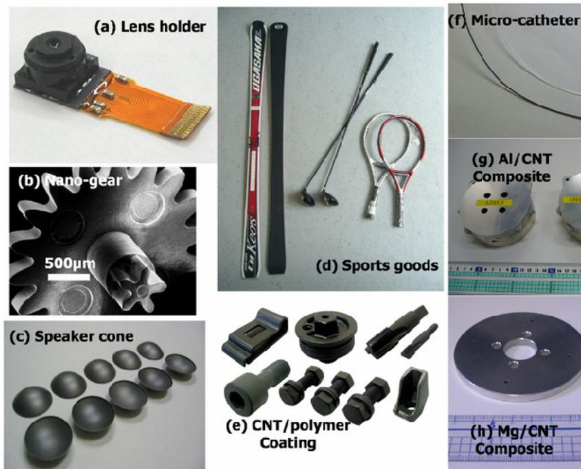
Figure 1 Various carbon nanotube-filled functional nanocomposites.
