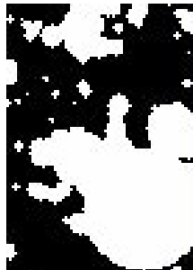
Figure 8: Fine detail section of pores simulating the morphological effects of radiolytic oxidation.
