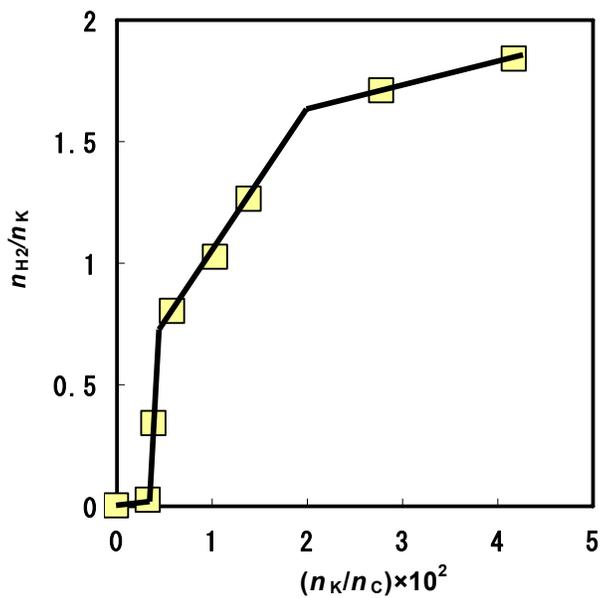
Fig. 2 Saturated sorbed amount of H<sub>2</sub>,  $n_{H_2}/n_K$ , at 77 K plotted against potassium concentration of K-GICs,  $n_K/n_C$ .
