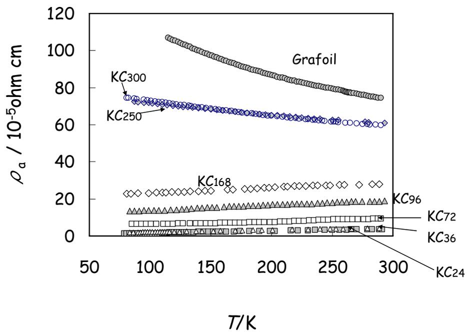
Fig. 1 Temperature dependence of electrical resistivity of K-GICs.
